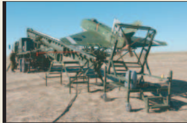
The Sperwer UAV at Suffield, Alberta this past summer after it had been hoisted onto the catapult ramp prior to launch.
