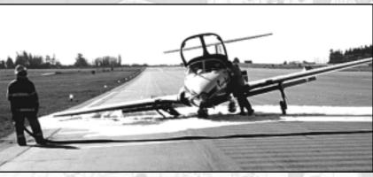
The damage sustained by aircraft #5 occurred due to a hard landing after a bounced touch-down exacerbated by preceding aircraft jet wash and down wash.
