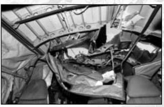
lodged in the roof of the aircraft. The port stub wing was dented by one of the thrashing aft rotor blades, but the fuel tank was not punctured.
