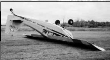
point. Immediately after that, the aircraft transitioned from wet to dry grass, and the sudden increase in traction on the locked wheels caused the tail to rise. Before the pilot could release the brakes, the aircraft was pitching forward. The combination of no headwind, low speed and low engine RPM provided no elevator authority to keep the tail on the ground.
