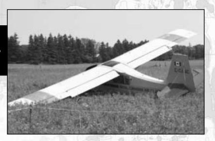
workers, without a corresponding increase in power. This allowed the airspeed to decay and induced a stall in close proximity to the runway. The resulting high sink rate on ground contact subjected the left landing gear to loads in excess of the design limits.
