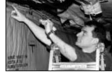
ed Non-Destructive Testing to confirm the length of the cracks. One was found to be a total length of six inches, while the other one was two inches. A survey was then conducted on aircrafts #306, #308, and #317, which also confirmed cracks of varying sizes and lengths.
