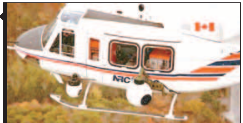
Enhanced Low Light Visible and Infrared Surveillance System.
