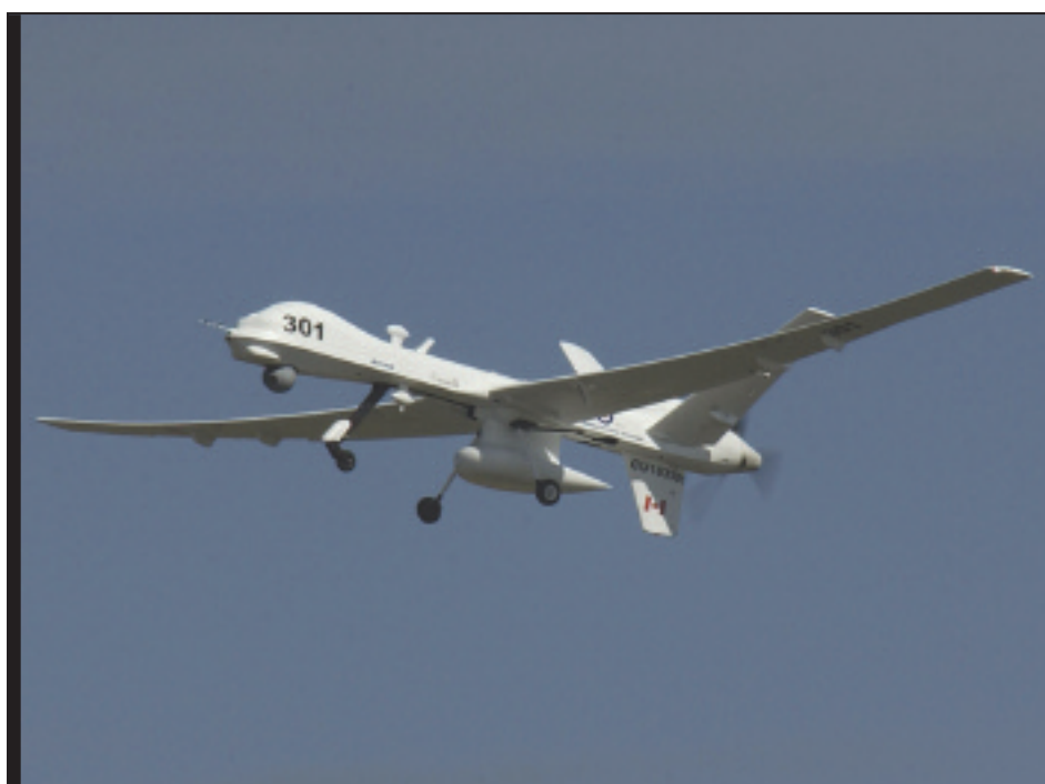
The Air Force played a key role in another world first last August when the CF flew an unmanned aerial vehicle (UAV) over domestic airspace during Ex NARWHAL. Here, Altair CU-163301, a medium-altitude, long-endurance UAV, takes off for a test flight at 5 Wing Goose Bay.
