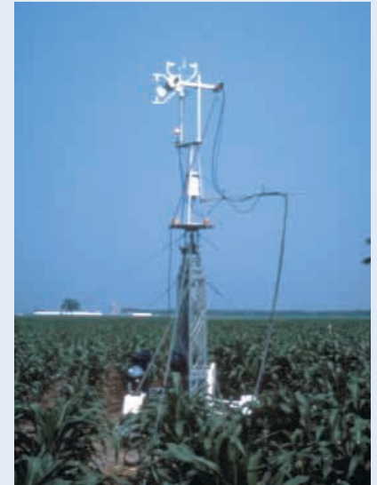
Tower-based system for measuring gas exchanges.
