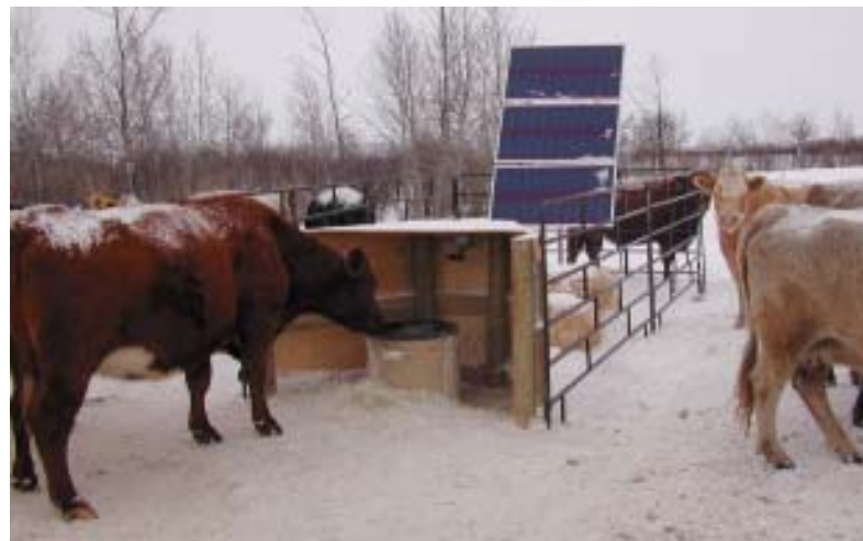
This motion detection watering system pumps water into a basin as livestock approach
