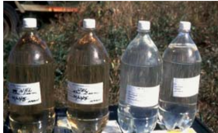
Alum coagulation greatly improves the clarity of water which allows disinfectants to work much more effectively
