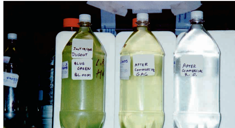
These bottles show algae passing through the primary GAC treatment system. Fortunately, the add-on RO unit delivered better water to the kitchen tap
