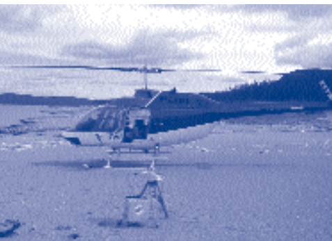
The Canadian Geodetic Service uses high-accuracy gravity and GPS observations to improve the "geoid" reference for elevations, aimed at providing GPS users with access to elevations.
