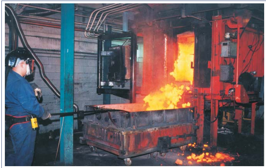
Discharging of metallurgical coke from CETC moveable-wall pilot oven
