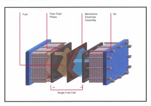
When many MEAs are stacked in series, the power of the cell becomes sufficient to support a large electric load such as a motor.
