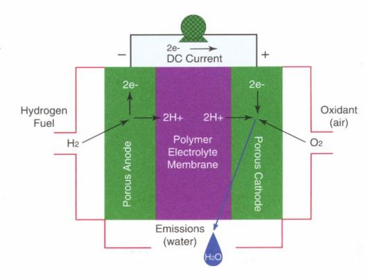
car or power a factory. Fuel is stored in a separate storage tank, just like gasoline. Oxygen from the air is used as the oxidizing agent – unlike in batteries, where the oxidant is chemically stored within the battery itself.
