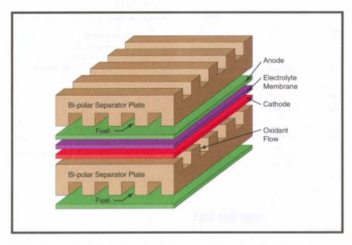
Single cells are stacked back to back in series electrically by means of bi-polar plates. The plates connect the anode of one MEA to the cathode of the next.
