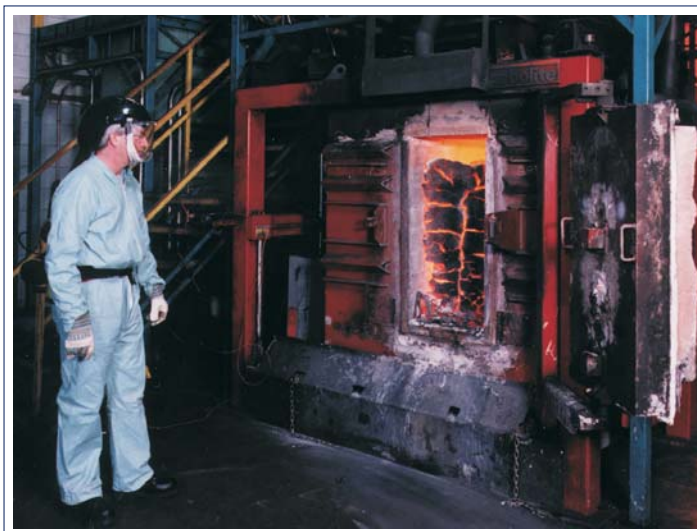
Pushing Coke from Slot Type Coke Oven
