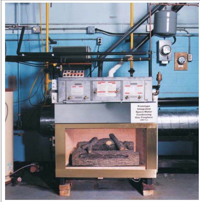
Prototype Integrated Space-Water Condensing Gas Fireplace
