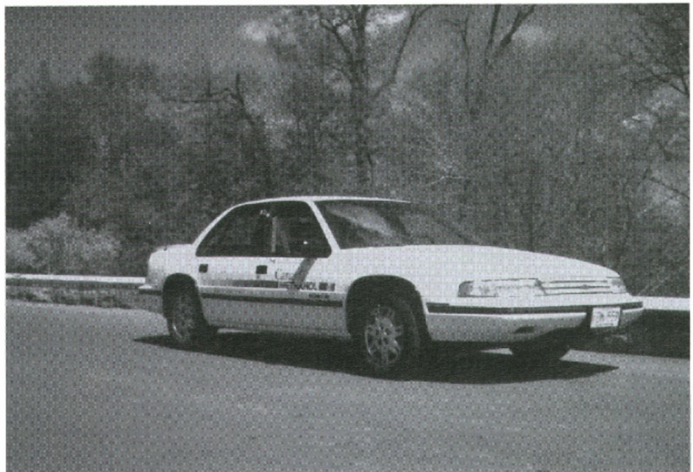
CANMET's variable fuelled methanol/gasoline Lumina.
