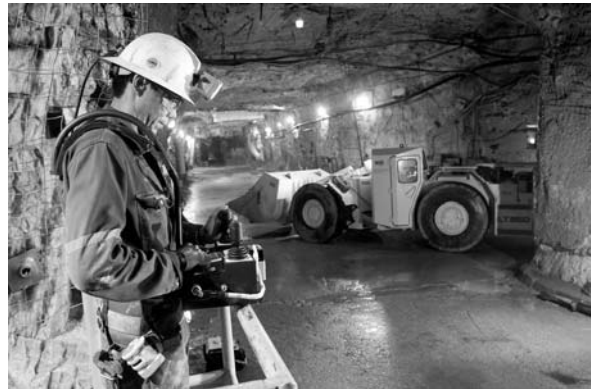
Canadian mining continues to innovate and automate to maintain its international competitive edge. The remote-controlled scoop tram shown here is being used to collect and transport uranium ore 640 metres underground at the world's highest-grade uranium mine at McArthur River, Saskatchewan (photo courtesy of Cameco Corporation).
