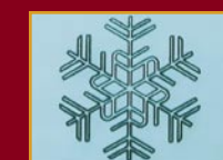
Fig. 1 Complex microchannel pattern on glass Diameter - 1mm and Channel width - 10 micron
