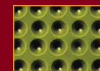
Fig. 2 Micromachined dents on glass with optical surface quality
