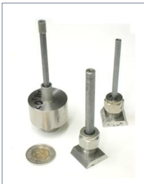
Figure 2: Vanadium cans used for containing powder samples
