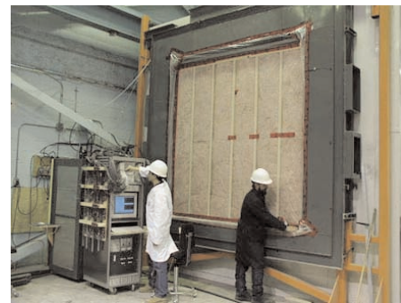
IRC researchers prepare full-scale wall specimen for an experiment in the Envelope Environmental Exposure Facility (EEEF)
