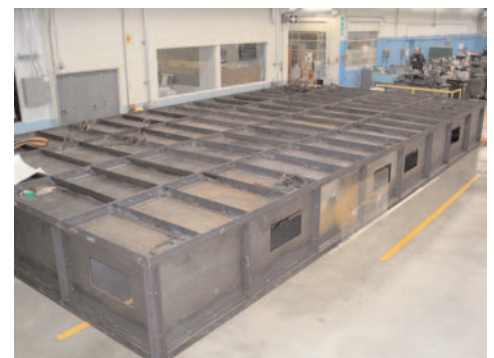
New 16' by 32' table for Phase IV investigation of wider roofing membranes
