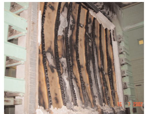
A wood-stud wall buckles during a fire test.
