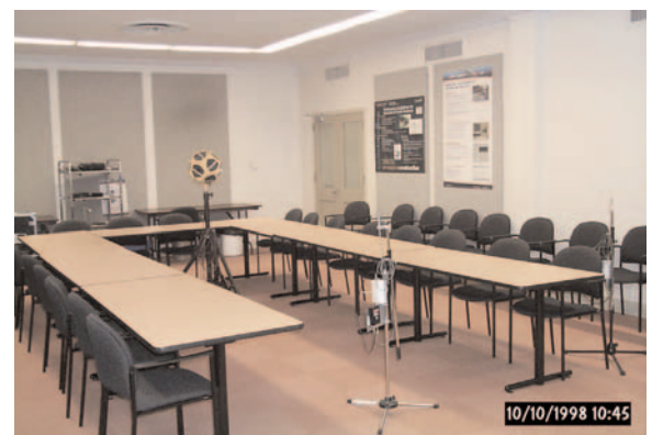
Acoustical measurements help characterize speech privacy issues
