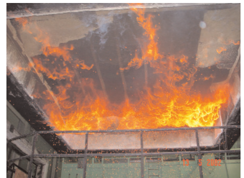
One of 60 floor assemblies, typical of those used in residential construction, undergoing a full-scale test at IRC
