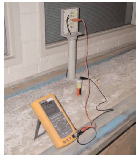
Reference electrodes are tested in high resistivity sand box
