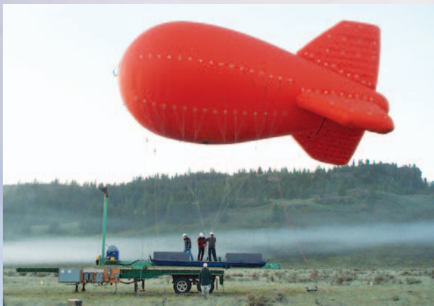
The Universe According to Bob — An inflatable aerostat nicknamed “Bob” is at the heart of an innovative Canadian design being proposed for the next generation of radio astronomy equipment. Known as the Large Adaptive Reflector, work is being carried out by the NRC Herzberg Institute of Astrophysics in Penticton, B.C.
