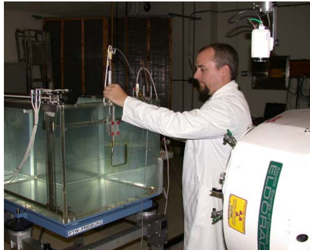
Brad Downton carries out commissioning measurements on the Co-60 irradiator after the replacement of the source.
