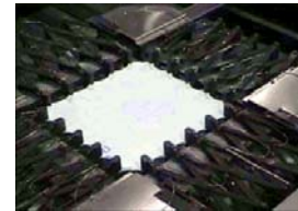
Biaxial sheet stretcher
