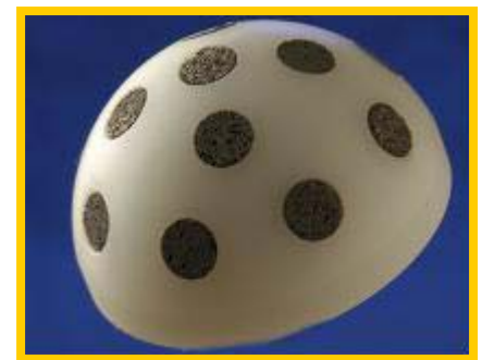
Prototypes of porous Ti attachment systems for dental implant (coating) and acetabular cup (inserts)
