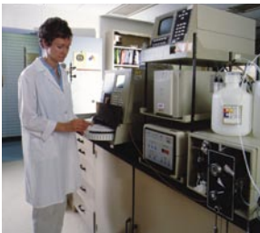
Chromatograph system used to characterize barley carbohydrates and proteins
