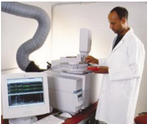
Using gas chromatography to analyse for mycotoxins
