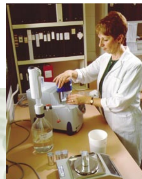
Determining sprout damage in wheat
