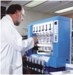
Measuring oil content by solvent extraction
