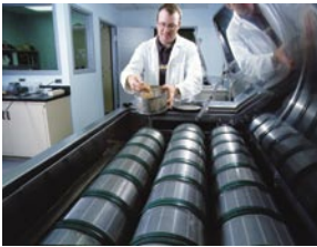
A micromalting system in the Applied Barley Research laboratory
