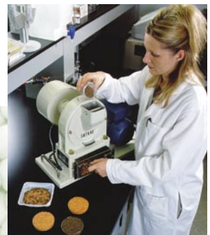
Evaluating the efficiency of methods used to hull red lentils
