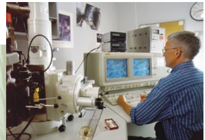
Scanning electron microscopy of biochemical changes in barley during malting
