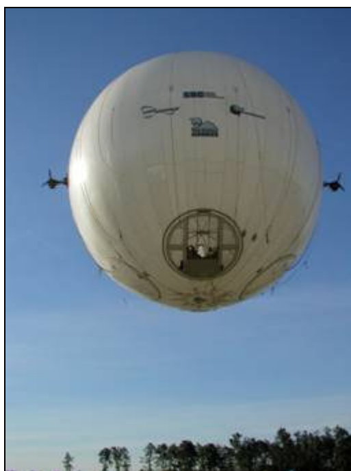
Figure 57. Spherical Airship. Source: Isopolar Airships
