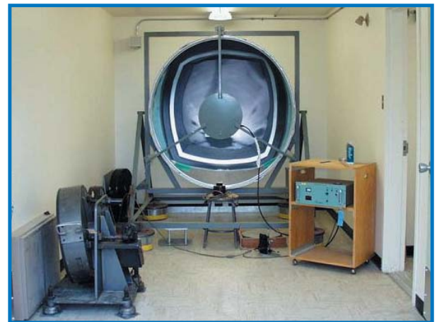
A 1.5-m diameter parabolic mirror for use as an active source for the 5.7-km long path
