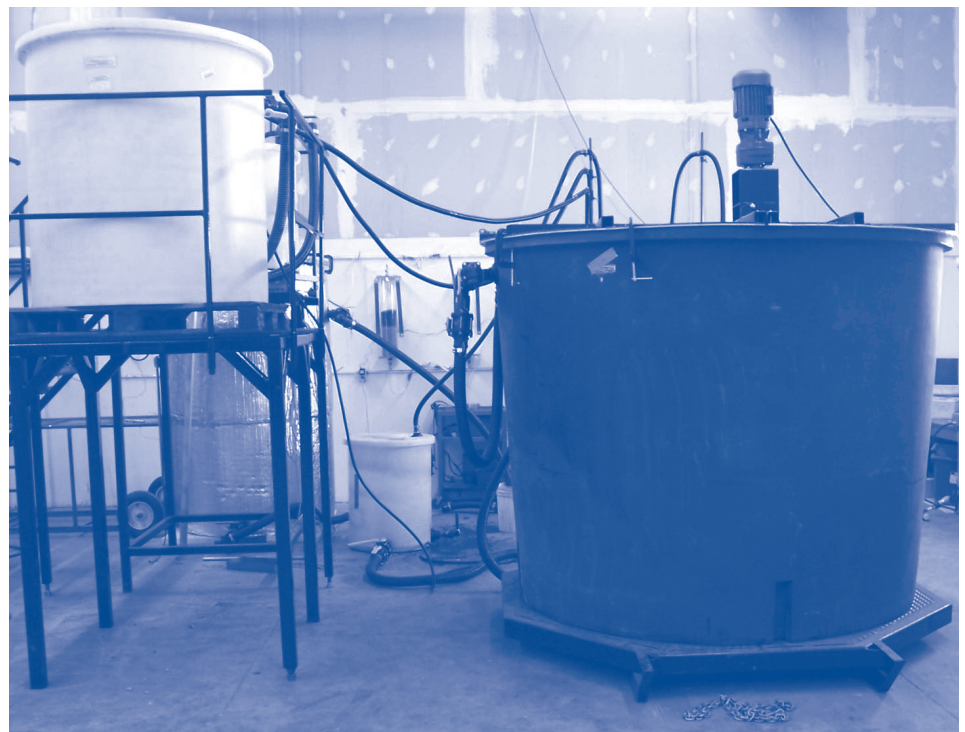
PAMI biodigester system with silver biodigester in the background. PHOTO COURTESY OF PAMI
