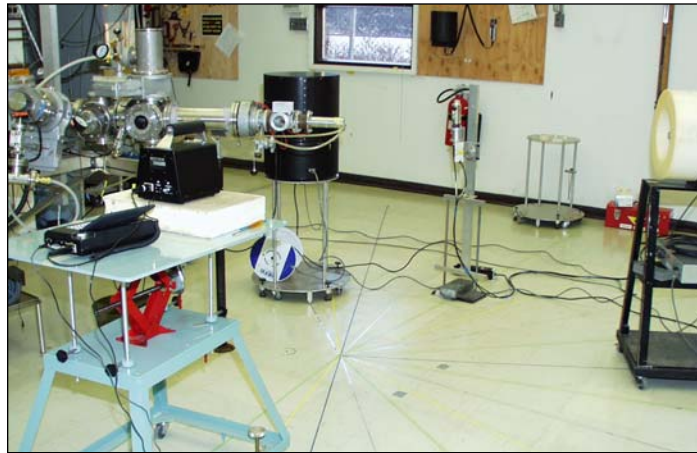
Van de Graaff equipment under test at angular beam energies with reference long counter at 0°.
