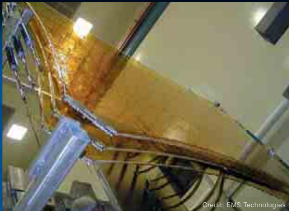
Membrane Synthetic Aperture Radar antenna under development at EMS Technologies, Ste-Anne-de-Bellevue, Québec.
