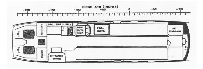
Figure 2.1 Cabin Dimensions (Plan View)
