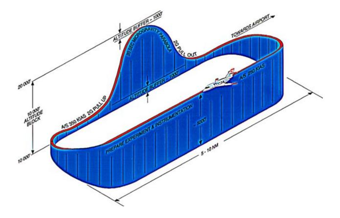
Figure 1. 1 Typical Microgravity Flight Trajectory
