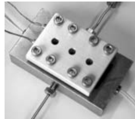
Single channel multiphase microreactor for solid catalyzed gas-liquid reactions
