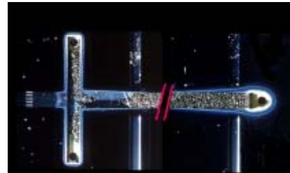
Single channel multiphase microreactor for solid catalyzed gas-liquid reactions
