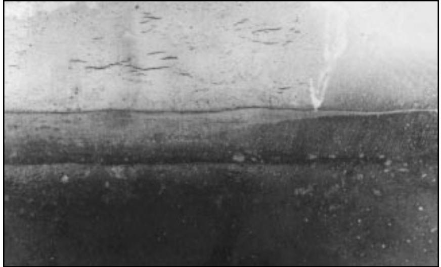
Figure 3.11 SCC cracks along and at the toe of longitudinal seam weld
