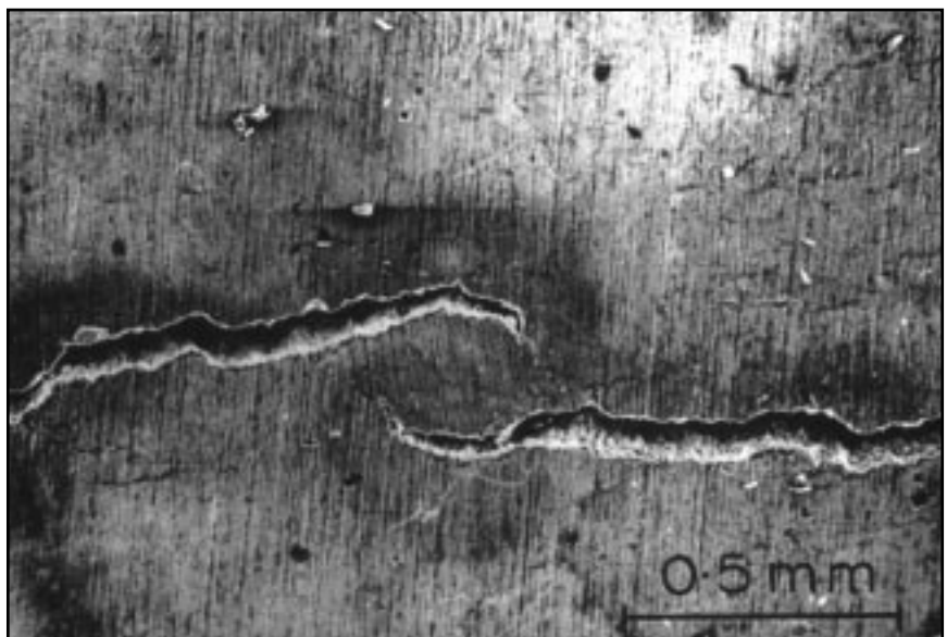
Figure 3.26 Cracks approaching coalescence
