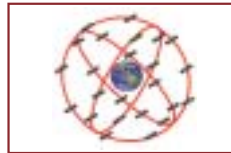
Figure 3: Navigation satellites in medium-Earth orbit (MEO), such as GPS, Glonass and the new Galileo system
