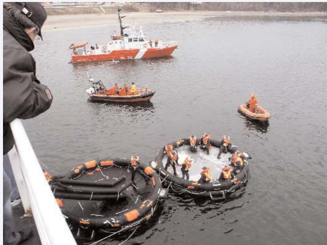
Evacuation chutes and life rafts are tested as crew and 'passengers' abandon ship.
