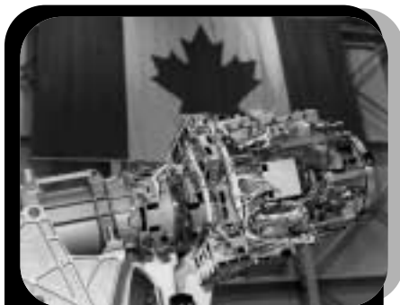
Detailed view of a component of Canada's Mobile Servicing System for the International Space Station undergoing testing at the Canadian Space Agency David Florida Laboratory in Ottawa.
