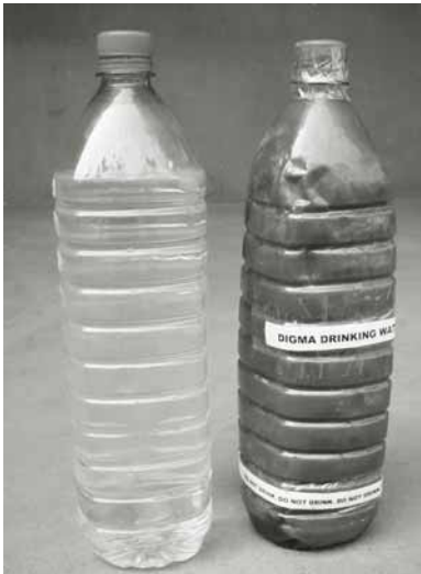
Water from a treated system (left) and community drinking water (right). Digma, Northern Region, Ghana.
