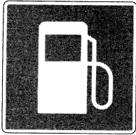
6.4.4 Gasoline station To indicate the location where motor vehicles may be refueled.
