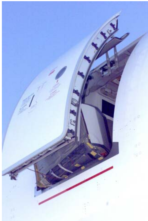
Figure 6 - Door L3 Jammed
