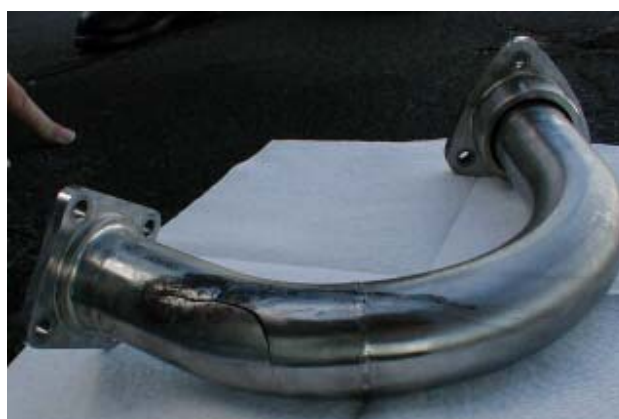
Figure 4 Fuel Pipe Crack & Scratches
