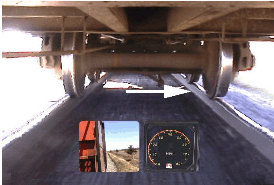
Photo 2. Test run image showing wheel lift at 60 mph
