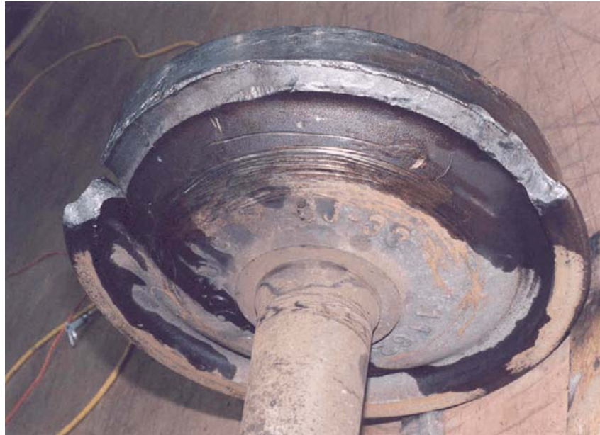
Photo 1. Fracture of rim of wheel L-3 of car DTTX 25029
