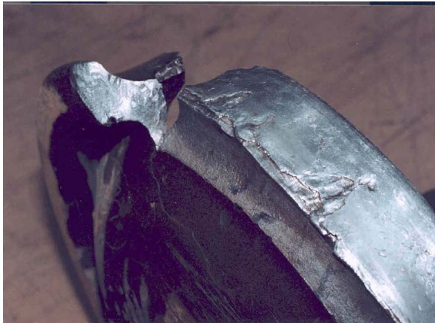
Photo 2. Shelling on the running surface
