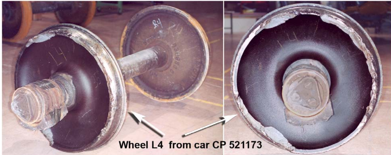
Photo 2. Broken wheel from car CP 521173
