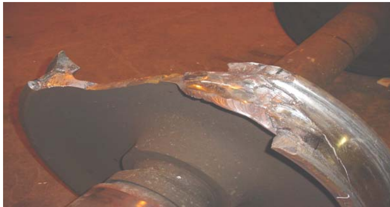
Photo 4. Broken wheel from car CNWX 111231
