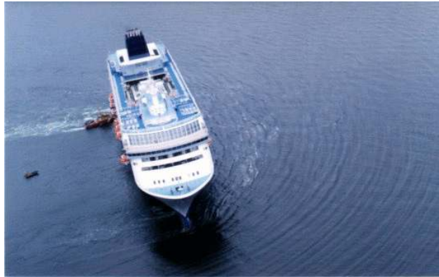
Photo 2. Norwegian Sky aground. Note current pushing the vessel against the Bancs de l'île Rouge
