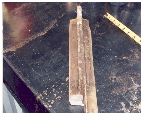
Figure 4. Horizontal fracture of the rail web
