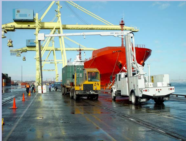
Canadian Border Services Agency officers use the mobile VACIS unit to scan a shipping container at the Port of Montreal.
